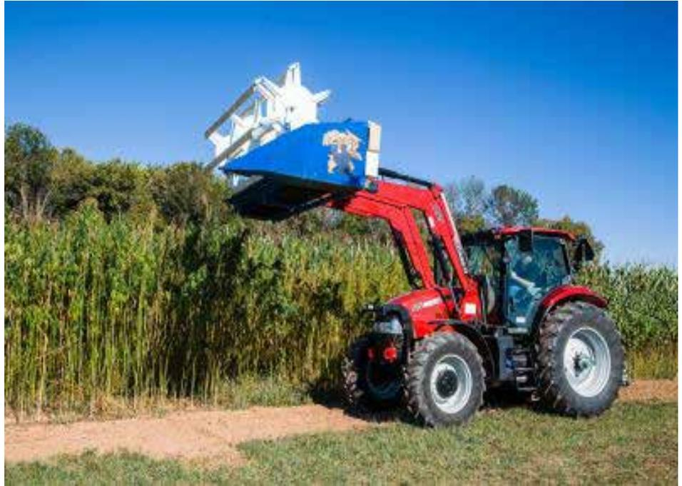
"Most implements use hydraulic power, but that would have made it harder to move from tractor to tractor," Stombaugh said. "We put a generator on the back of the tractor to create power for the harvester. All of the equipment can fit on the back of a gooseneck trailer, so it's very easy to move from one machine to another."
